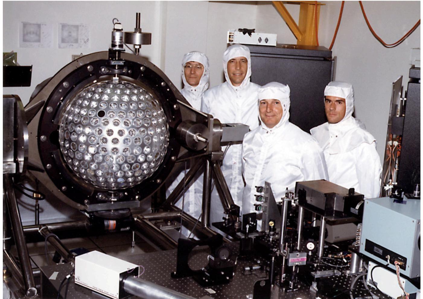
LAGEOS-2 at NASA/GSFC for optical testing
